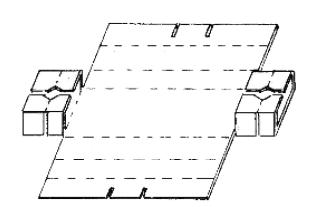
Form both end panel into box shape as shown.
