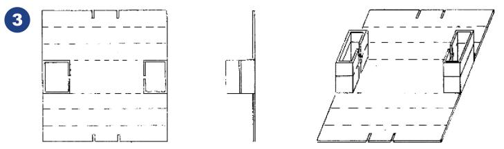
Tape box shaped ends from Step 2 and fold up 90 degrees until inside of box is flush with cover sheet, as shown.
