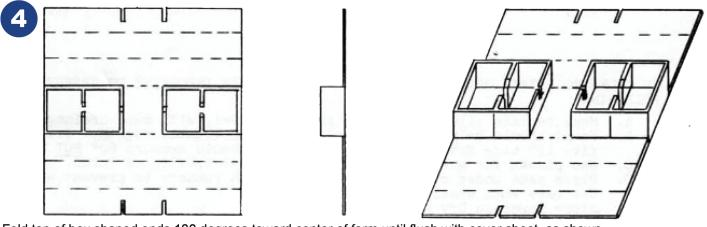
Fold top of box shaped ends 180 degrees toward center of form until flush with cover sheet, as shown.
