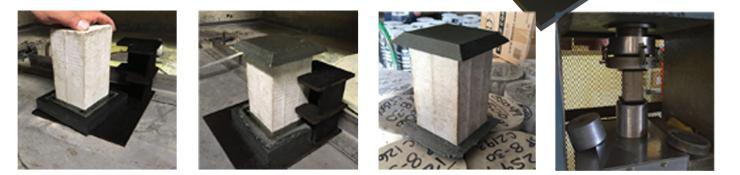
•Vertical capping guides help ensure samples remain perpendicular during the capping procedure. No more need to use a level or seat specimens by eye.
