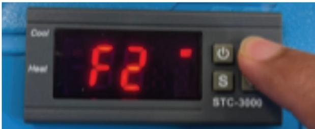
Repeat same procedure as Step 1 to set desired temperature difference value. This value will indicate how much variation from set temperature is allowed before compressor or heater starts to maintain the set temperature F1.
