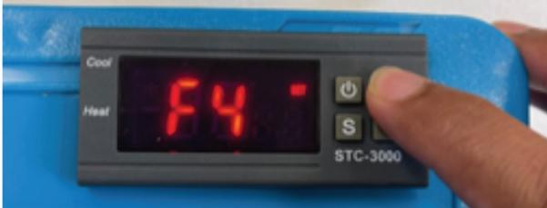
Repeat same procedure as Step 1 to set temperature calibration value. It is set to 0°F initially.
