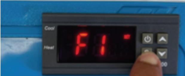
Step 1: Press and hold "S" and simultaneously hold "up" then "up" or "down" to set desired temperature value as shown in picture below. Once desired temperature is set, release both "S" and "up" or "down" button.
