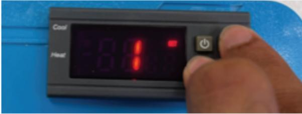
Press “up” button to navigate to F4 as shown in picture below.
