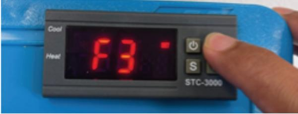
Repeat same procedure as Step 1 to set compressor delay time before cooling begins.
