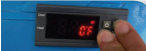
Press “up” button to navigate to F5 as shown in picture below.
