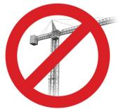
The lifting strap is only to be used to remove the concrete from the pans. The strap is not to be used to lift by crane or be flown. Any lifting of the pan to an elevated location needs to be done using a forklift and lifting from the bottom of the pans.
