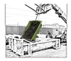
Put the forks through the attached sling and raise the pan upward. The patented design allows for the pan to lift vertical past 90 degress to allow for the concrete to be ejected from the pan.
