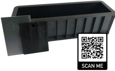
Use the Deslauriers **4" PLASTIC BEAM MOLD** to cast concrete for flexural strength testing. This durable one-piece mold is constructed from heavy duty plastic and engineered with reinforcing ribs.
