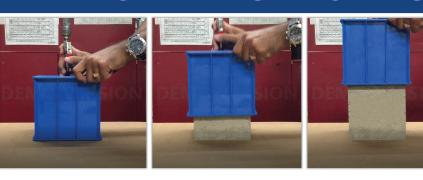
Specimen removal is simple, fast and easy. Just remove the plug from the hole in the bottom of the mold and apply compressed air to the hole. The mold will slide right off the hardened specimen.
