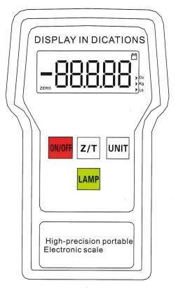
ON/OFF: Press to power on press to power off
